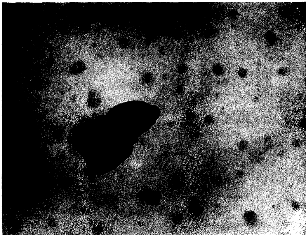
FIG. 3. Electron micrograph of Rh/Al 2 O 3 catalyst, magnification 240,000 \times .
