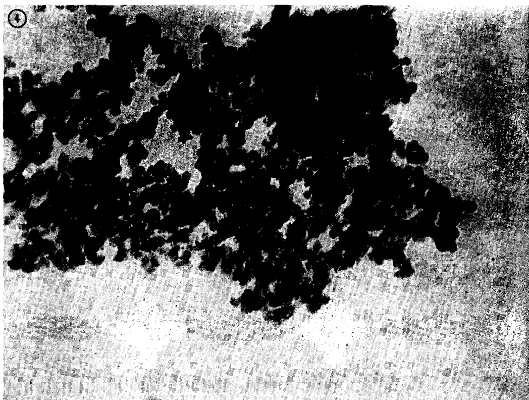
FIG. 4. Electron micrograph of Rh/SiO 2 catalyst; magnification 248,000 \times .
